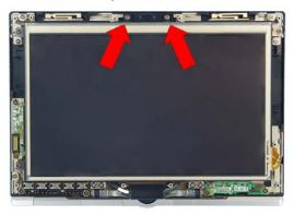
7. Extract 2 screws from the display latch and lift it out.
