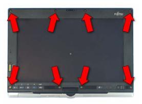
9. Press the front cover into place and secure it with 8 screws.
